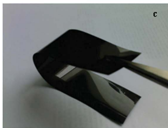
Figure 3 Mechanical properties of neat PEN and PEN/GNs composites: (a) tensile strength and modulus, (b) elongation at break, and (c) photograph of PEN/GNs composite film with 5 wt % GNs content (length: 15 cm, width: 5 cm, and thickness: 85 μm). [Color figure can be viewed in the online issue, which is available at wileyonlinelibrary.com .]
